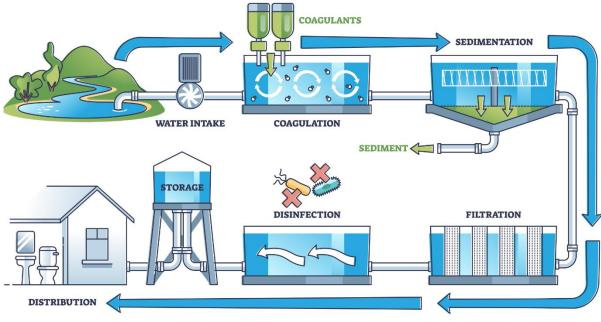
Figure 1 Typical Water Treatment Process for Drinking Water
