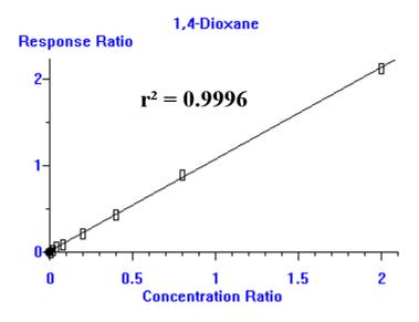
To verify that the 0.5 ppb calibration point is precise and accurate, a reproducibility test was performed. Seven duplicate samples were prepared at 0.5 ppb. An example of a SIM scan for 1,4-Dioxane at 0.5 ppb is displayed in Figure 2. These seven duplicate samples were analyzed to establish a minimum detection limit (MDL) for 1,4-Dioxane. The reproducibility and MDL results can be found in Table III.
