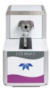
The closed-system is flushed continuously with 200 cc/min of carrier gas. Once oxidized, the sample exits the LSS and is carried to the Lotix TOC Analyzer's Non-Dispersive Infrared Detector (NDIR) for analysis. The signal from the NDIR is integrated by the TOC TekLink software and displayed as analytical results in ppmC or µgC/g concentration units.
