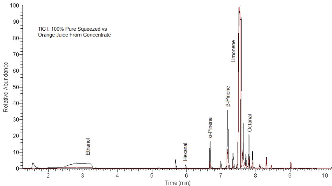
Figure 9: TIC overlay of 100% pure squeezed (black) compared to orange juice from concentrate (red).
