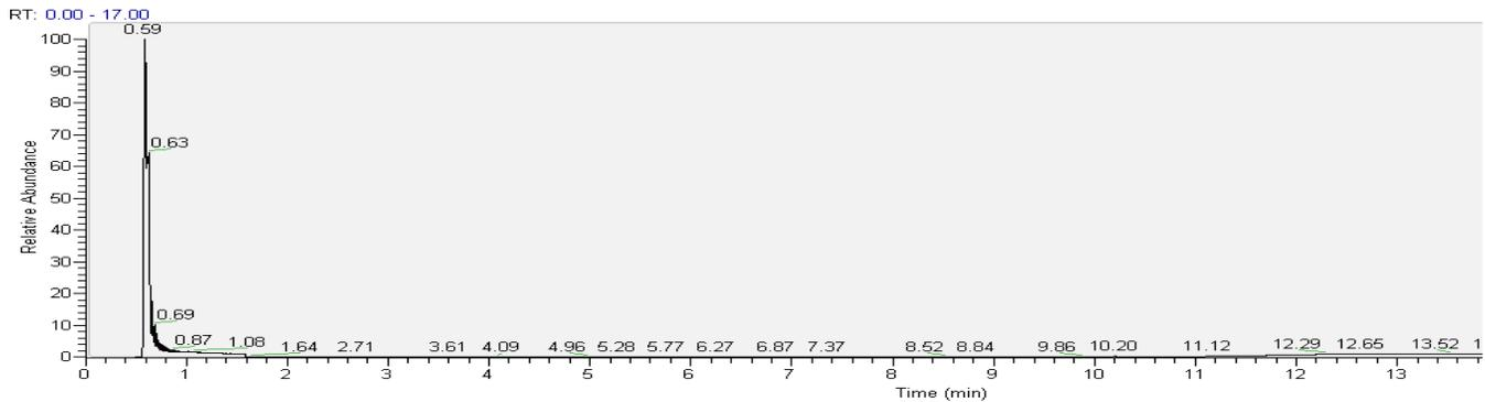
Figure 2: Typical blank run prior to each analysis
